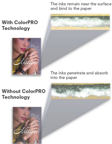
FIGURE 1: ColorPRO Technology is incorporated into the paper-making process, delivering visibly enhanced print quality when used with HP pigment inks
